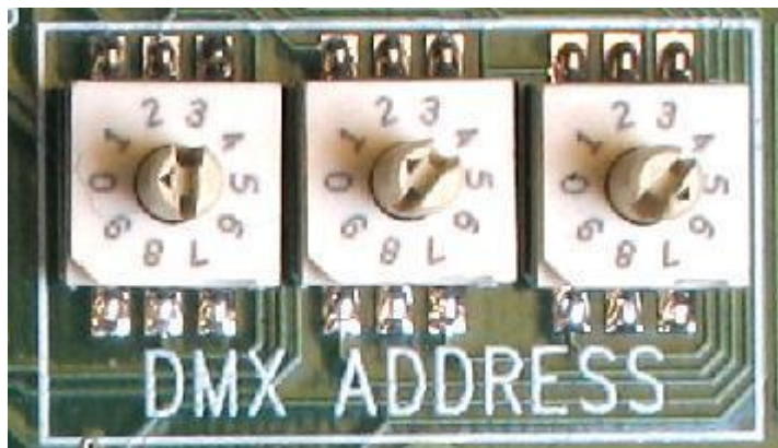
EXAMPLE DMX ADDRESS SET TO 016 NOTICE THE POINTER ON THE SHAFT
