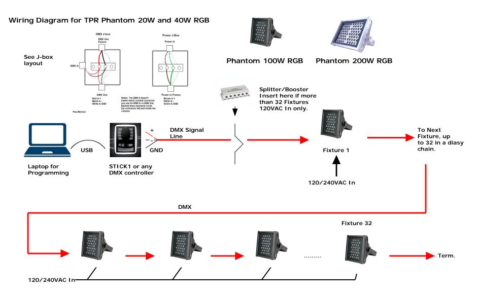
Notes: From the DMX Controller to the last fixture in line you can run 1000' and 32 fixtures. If you go above 32 fixtures you must use the Splitter Booster (120VAC only). The Splitter Booster has an input (from the controller) and 6 outputs. Each output can have 32 fixtures and up to 1000' to the last fixture. For runs of over 20 fixtures we recommend a DMX terminator plug at the end. Red line is DMX cable- AWG18/3 or AWG18/2 with a shielded braid. Belden 88770 or 3105.
