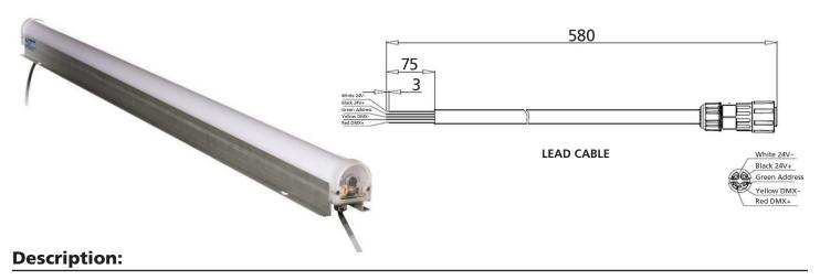
The **TPR Phantom™ Pixel Tube** is a rigid RGB fixture for Architectural and Entertainment use. It is available in 1′, 2′ and 4′ lengths, is IP65 rated for outdoor use, and is Pixelated for chasing color scenes. Each 6″ is a pixel. Each pixel can be programmed independently for color change, chase, etc. This fixture is run via DMX512 protocol and is extremely light weight and easy to install. Each 6″ is 3 channels. Example: 4ft=24 channels. Discuss control options with factory.
