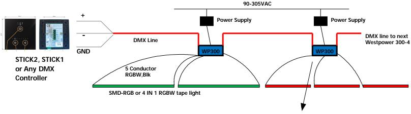
Notes: The Westpower 300-4 can handle either 12VDC or 24VDC. The White knobs on the board are for DMX addressing. When put to 000 it enables the Black Potentiometer knobs that will dim the Red, Green, Blue and White Channels.
