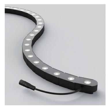
TPR Akrobat™ Flexible LED Wall Grazer is designed to provide high quality illumination for columns and curved architectonic surfaces, with a variety of lens options that can be used for flood lighting, wall grazing, wall washing and accent lighting. This product is IP67 and operates on 24VDC. 4 meters can be connected end to end (13.12')
